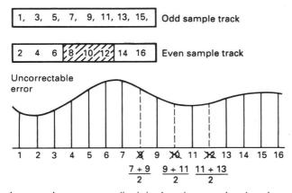
In cases where error correction is inadequate, concealment can be used provided that the samples have been ordered appropriately in the recording. Odd and even samples are recorded in different places as shown here. As a result an uncorrectable error causes incorrect samples to occur singly, between correct samples. Therefore an approxiamtion of the existing values are taken via the process of interpolation.
