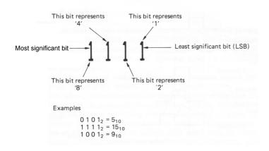
The word length of a digital device becomes the measure of the "Resolution" of the system and with digital audio better resolution means better fidelity of reproduction. (24 bit systems are superior to 16 bit systems)
