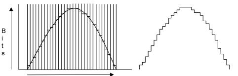
According to the Nyquist theorem, S samples per second are needed to completely represent a waveform with a bandwidth of S/2 Hz, i.e. we must sample at a rate which twice the highest through put frequency to achieve loss less sampling. Therefore for a
